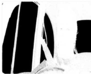
Screen Gain = 150 giving background show through and over eroded edges.
